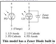
This model has a Zener Diode built in as a protection circuit against static electricity.
