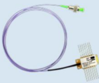
butterfly package with single mode fiber, TEC and NTC, FC / APC connector
