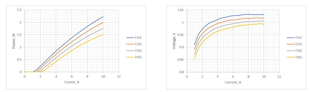
Typical operating current: 7A Typical operating power: 1.3W Maximum current: 10A Maximum power: ~2W Voltage: <1.2V
